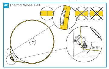
If the unit contains a thermal wheel heat exchanger, please ensure that the rotation sensor is aligned with the sensing studs, as this can become misaligned during transport / installation thus causing a fault signal.
