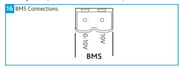
Reversal of the BMS connection will damage the control.
